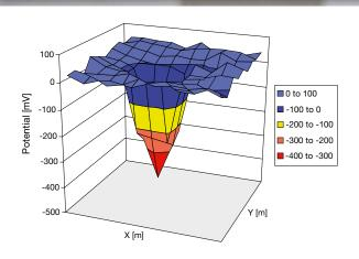
The electrical potential distribution over a corroding area can be represented as a "funnel" centered on the anode, whose shape and extent is defined by the actual ongoing corrosion as well as by the concrete electrical resistivity
