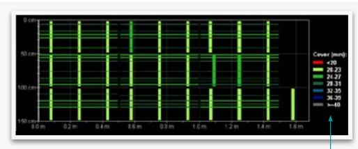
Tap on the screen to switch between Cover, Diameter and Signal Strength View
